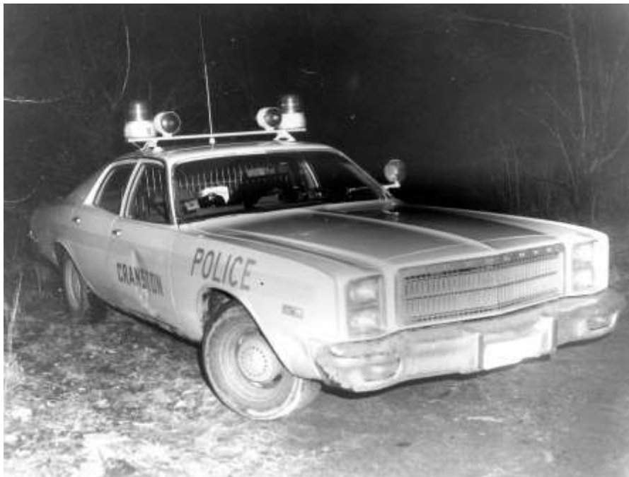
A 1978 Plymouth, Note the long "whip" antenna on the roof.
