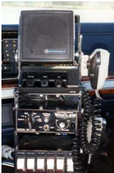
A ‘radio tree’ set-up, first introduced in the 1991 Fords. The radio, public address, lights and siren controls were all within easy reach.
