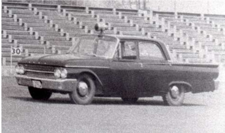
A 1961 Ford used by Patrolman Bill Loux of the K-9 Division. The car was black with no markings. (Note the combination red light/siren on the roof.) This vehicle had a six cylinder engine with 3-speed shift on the column.
